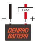
c. Put the fuse between battery and inverter on the positive side. The LED in front of grounding terminal will show red if reverse polarity, please correct the wiring again.
